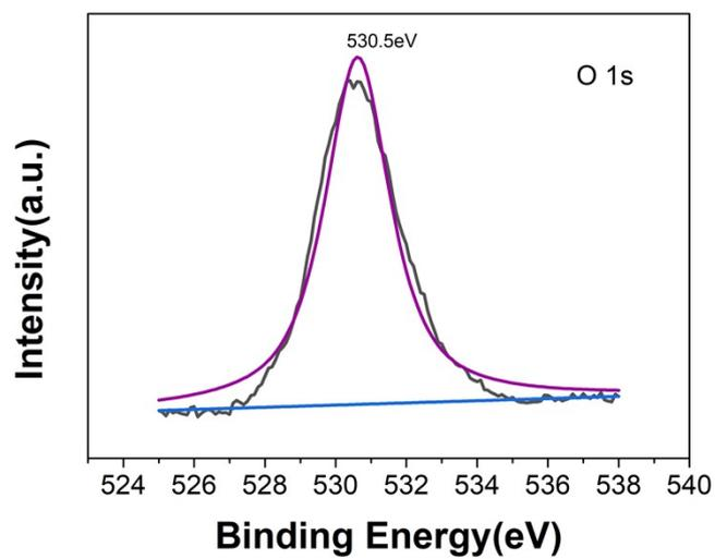
**Figure S3.** High-resolution XPS spectra of O 1s for the Nb<sub>2</sub>O<sub>5</sub>.
