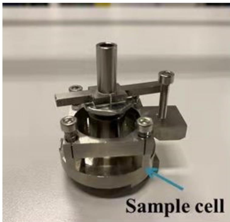
**Figure S10.** The quasi-operando XPS cell used in this work.
