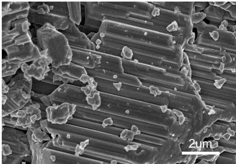
**Figure S2.** SEM image of commercial Nb<sub>2</sub>O<sub>5</sub>(c-Nb<sub>2</sub>O<sub>5</sub>).
