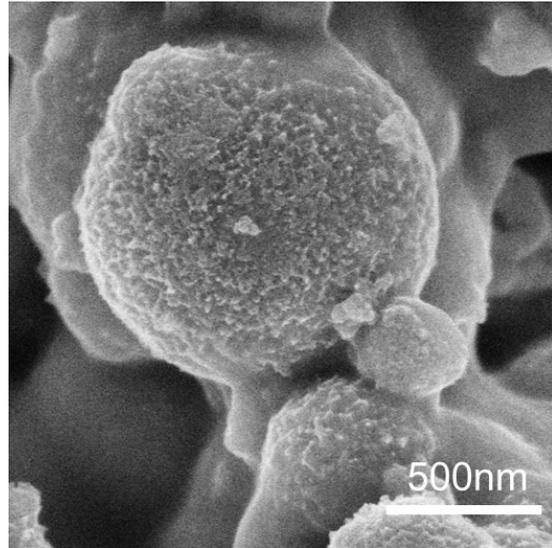
**Figure S7.** SEM image of the NbO<sub>x</sub> after electrolysis.
