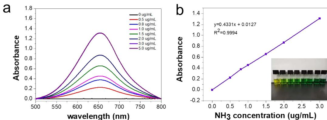
**Figure S5.** a) UV-Vis absorption spectra of indophenol assays with various  $\text{NH}_3$  concentrations after incubated for 2 h at room temperature. b) Calibration curve used for calculation of  $\text{NH}_3$  concentrations.
