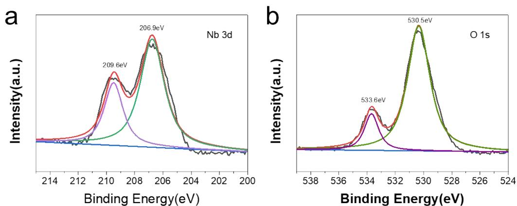
**Figure S9.** XPS spectra in a) Nb 3d and b) O 1s regions of Nb<sub>2</sub>O<sub>5</sub> after electrolysis.
