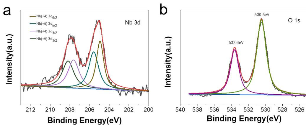
**Figure S8.** XPS spectra in a) Nb 3d and b) O 1s regions of NbO<sub>x</sub> after electrolysis.
