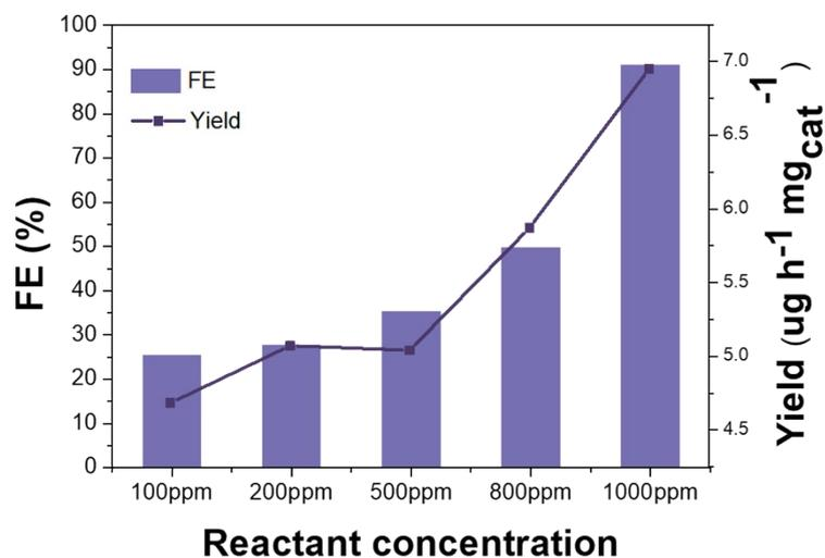
**Figure S6.** Potentiostatic tests were measured at  $-0.75$  V in the same electrolyte with the addition of different content of  $\text{NO}_3^-$  (100, 200, 500, 800, and 1000 ppm).
