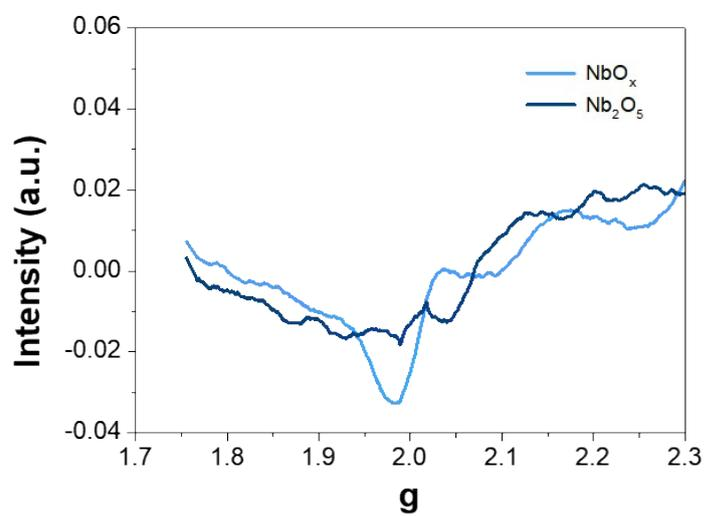
**Figure S4.** EPR spectra of NbO<sub>x</sub> and Nb<sub>2</sub>O<sub>5</sub>.
